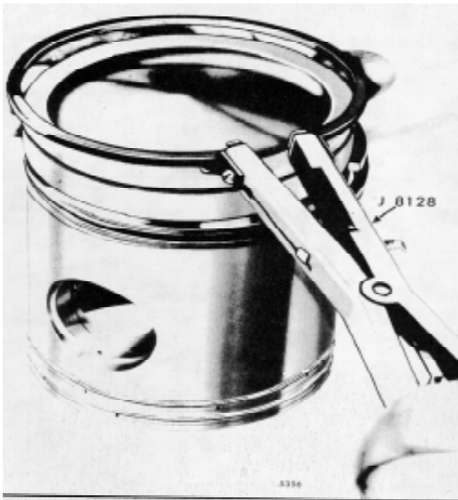
Fig. 16 - Removing or Installing Piston Rings
