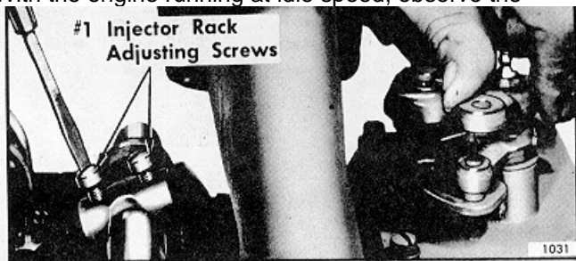
Figure 8 - Adjusting No. 1 rack to Governor
